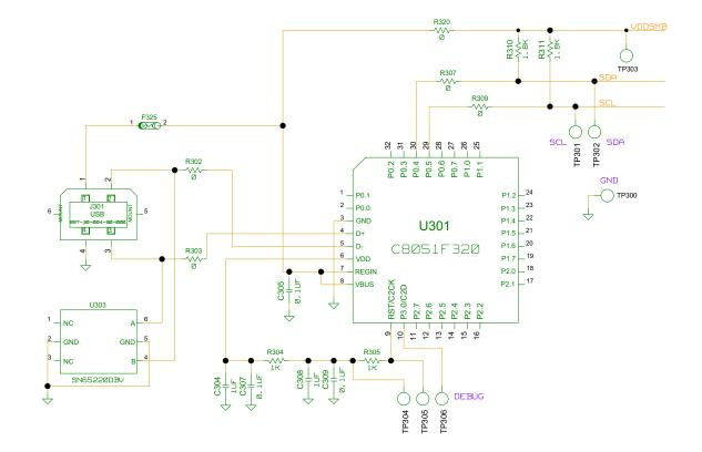
FIGURE 14. ISL88736EVAL1Z SCHEMATIC (USB - SMBUS INTERFACE)
